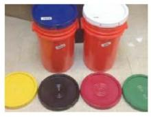
The actual bolt kegs (containers parts are shipped in) can be just as important. It is not recommended to store unprotected outdoors. Parts should be kept in weather tight kegs without seams to assure that moisture does not creep in. Some manufacturers are now shipping in Rigid Polyethylene Kegs, these containers can have a rubber gasket installed under the lid which creates a weather resistant seal. The lids on these types of containers make it
